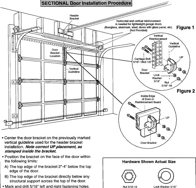
• Mark and drill 5/16" left and right fastening holes. Secure the bracket as shown in Figure 1 if there is vertical reinforcement.
